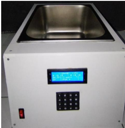
Gambar 5 Alat Water bath Dilengkapi Indikator Level Air Berbasis Arduino Mega2560
