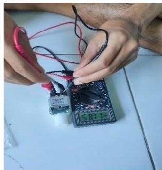
Gambar 6. Tegangan Solenoid Valve saat ON
