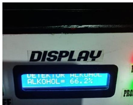
Gambar 3 Hasil Pengukuran Kadar Alkohol 70%
